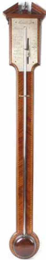
A George III inlaid mahogany stick barometer. The silver scale engraved 'Manteca, London N. 1780' (probably Dominic Manticha), reading from 28 to 31 inches of pressure, with vernier beside exposed mercury main tube, the trunk with brass urn finial and architectural broken pediment over chequered stringing to a turned cistern cover, 38.75", (98.5cm) high. £300-500 (plus 24% BP*)
